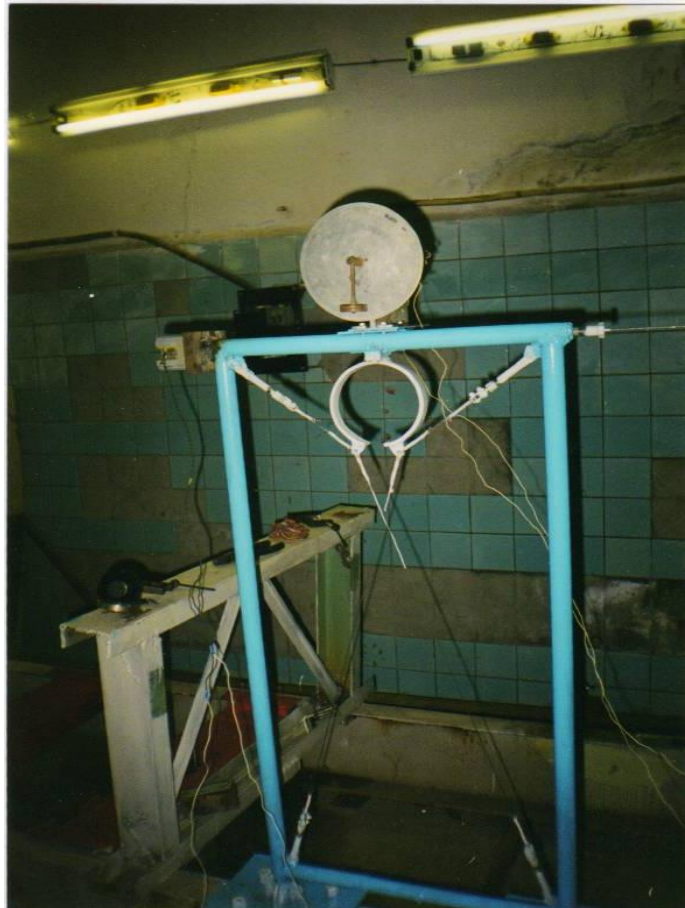
Fig. 20 View of experimental model of the frame with horseshoe-shaped bracing.
