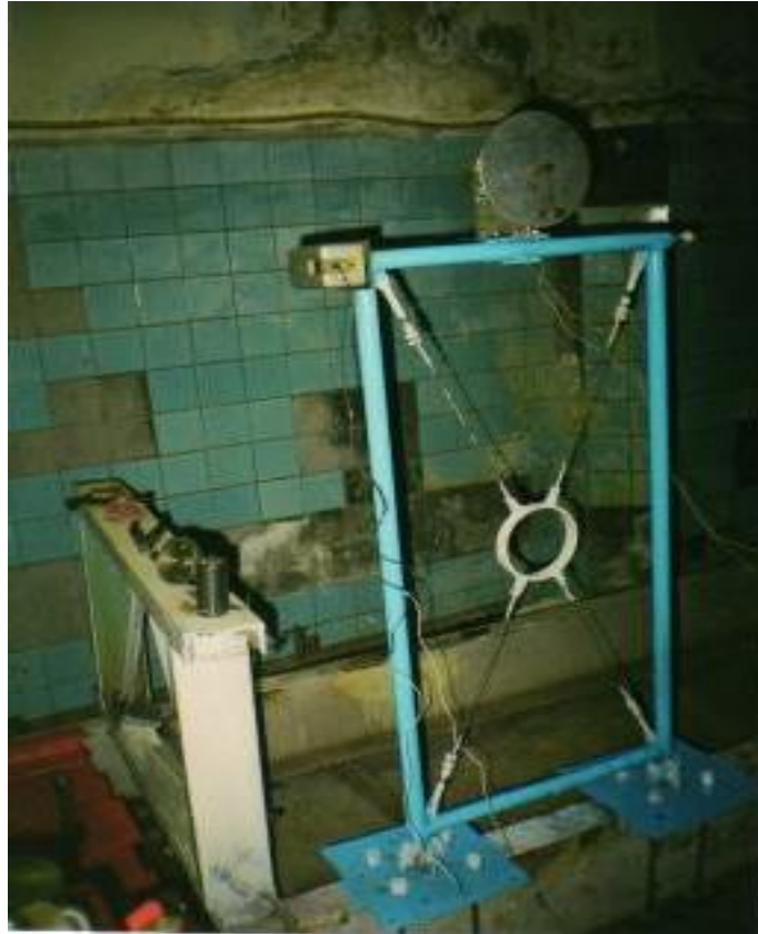
Fig. 18 View of experimental model of the frame with ring bracing.
